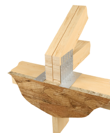
Typical SBP one tab up alternate installation
